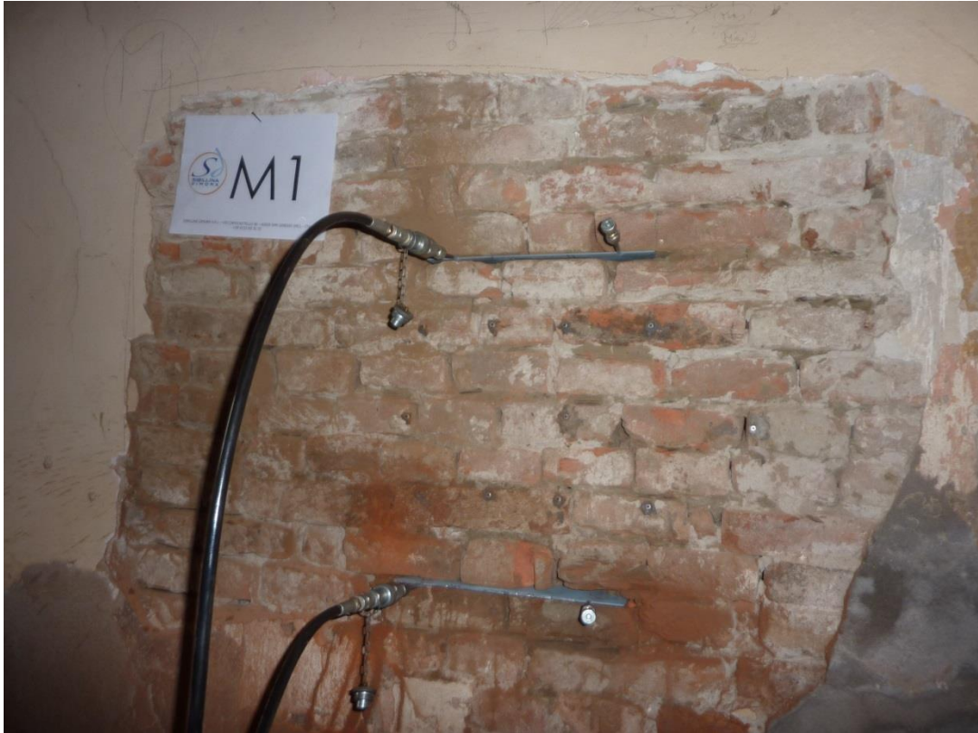
Figure 93. Double flat jacks test
