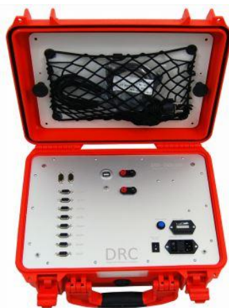
Figure 43-a. 8-channels DaTa500 acquisition system
