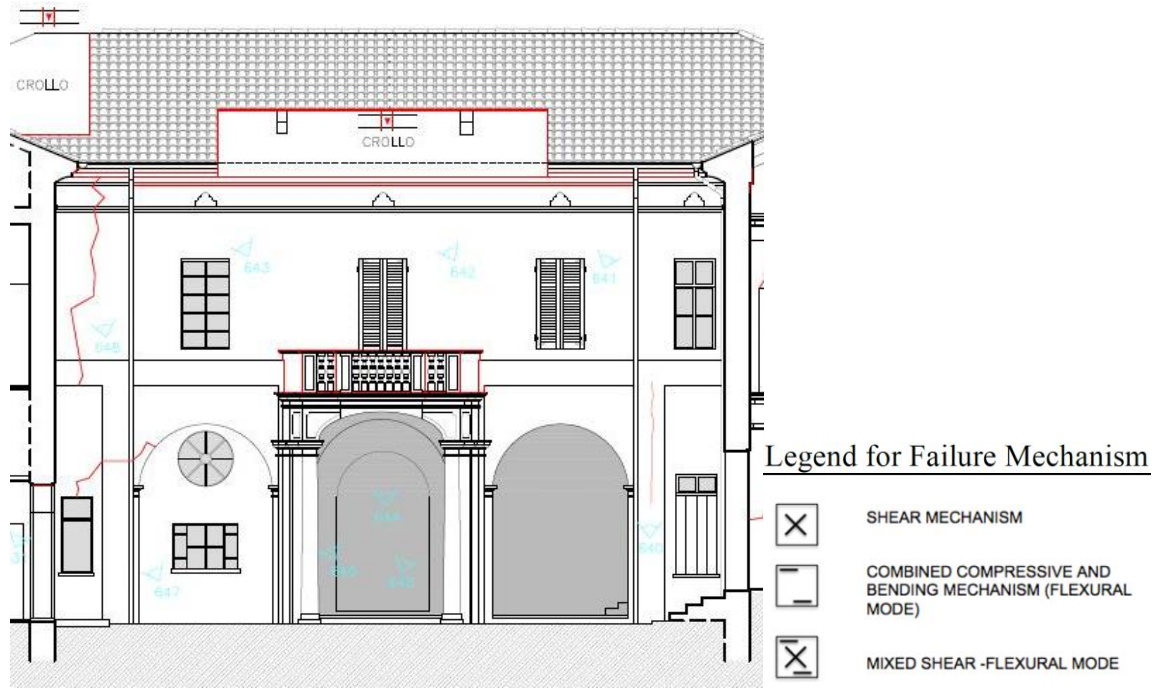
Figure 191. Seismic events 2012 in Emilia_ damage suffered by wall 4
